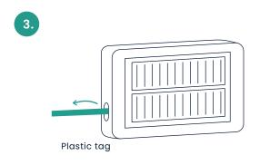
Pull the plastic tag completly out from the Theo device.
