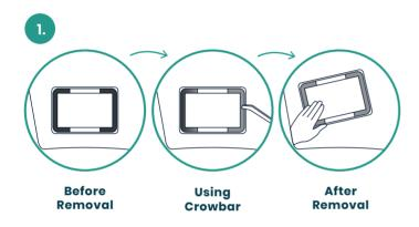
Remove the device from the windscreen using **the plastic crowbar provided**. Use the crowbar to edge the device off the windscreen.
