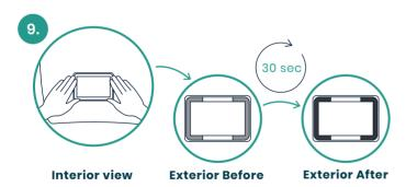
Theo should be readable from the inside to ensure your device is correctly orientated. In the same area you cleaned, press the device firmly against your windscreen from inside your vehicle.
