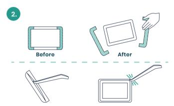
Place the narrow end of the crowbar into the gap between the device and the cradle, using the crowbar to leverage the device out of the cradle.
